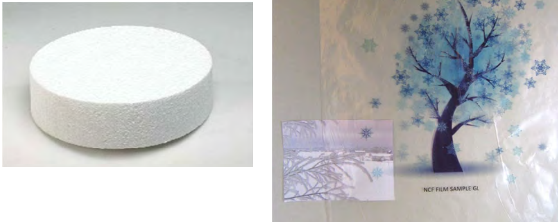
Figure 25. On the left, nanocellulose foam. On the right, printed film of nanocellulose manufactured in pilot scale through controlled adhesion, spreading and drying of NFC without any wiremarkings (VTT).
