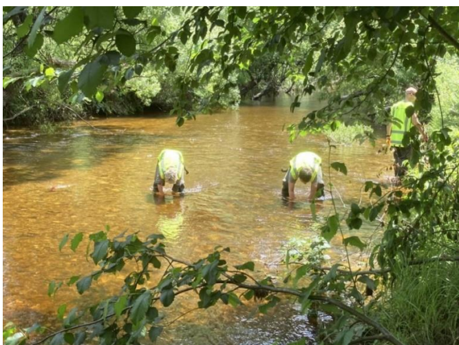
Figure 18. Donald Creek paired catchment study: Data collection for the study includes setting cotton strips to monitor bacterial and nutrients in the streams.
